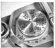
The required scale settings of the synchro-dial depend on the type of flash bulb used and on the shutter speed required. They are read off from the following table. (A copy of it is enclosed with every synchronized LEICA and can be slipped into the ever-ready case).
